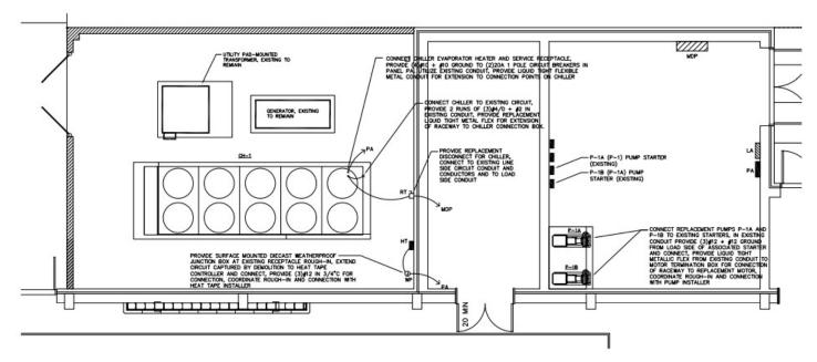
The 180 TR (Tons Refrigeration) chiller serving Rock Hill HS F-Building Gym suffered a compressor failure (1 of 2) in the spring of 2024. It is approximately 24 years old and repair components are not available which necessitates a complete unit replacement. Due to extended manufacturer lead times, the unit has been operating at 50% capacity with frequent periods of downtime resulting from unit faults and safety trips.
